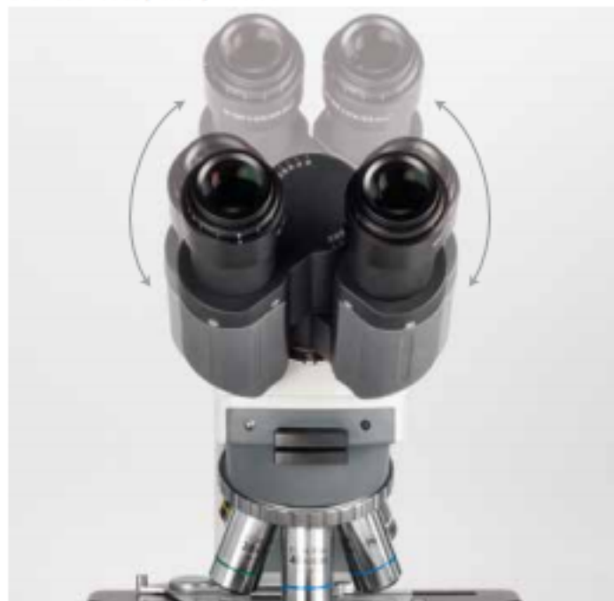
EYEPIECE TUBES | "Butterfly" movement
